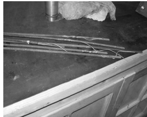
Fig.4 Strain gauges were installed on the bars
