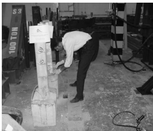
Fig.8 Cleanig surface of the damaged columns
